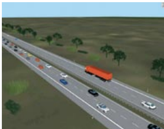
Realistic traffic and transportation modelling using VISSIM, for example, support transportation planning.
